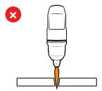
Torch height too high. Excessive bevel, plasma stream may not cut all the way through the material.
