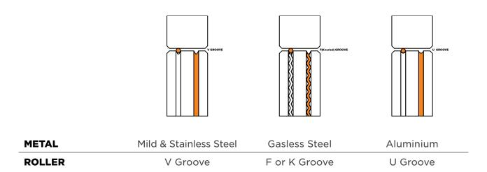
Each roller comes with two grooves; these are the wire sizes (e.g. 0.6mm & 0.8mm). You'll need to make sure the roller groove size is the same as the wire you are using. To replace a roller, unscrew the retaining cap and take the old roller off. Place the new roller on (lining up the keyway on the roller with the key on the machine) and re-screw the retaining nut.
