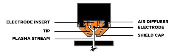
Plasma can cut through anything electrically conductive; steel, stainless steel and aluminium are all fair game. In comparison, oxy cutting will only work on metals that contain iron, as it works through chemical reactions, such as oxidisation (it's like a sped-up version of rusting) instead.
