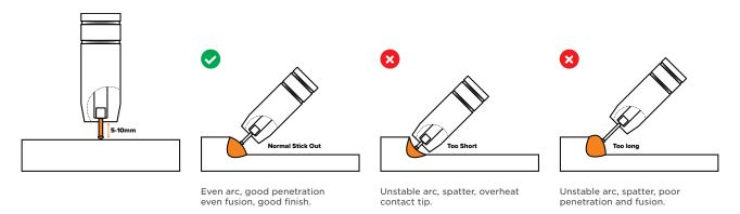
The first problem is that your feeding wire acts as a resistor, so the longer it is coming out of the torch and into the weld pool, the lower your machine will drop the amps, so it won't run as well. The second problem is that your shielding gas will no longer be able to reach your weld pool, and you'll increase the number of defects – like porosity – in your weld.
