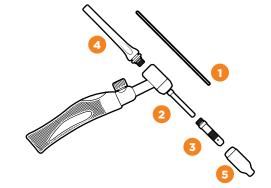
The collet and collet body should match the size of your tungsten (if your tungsten is 2.4mm thick, the borehole in your collet and collet body need to be 2.4mm wide).
