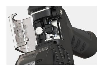
As well as your standard MIG torches, you can also get an aluminium specific torch, called a 'spool gun'. Spool guns are set up slightly differently than the MIG torches, as the wire spool is not connected in the machine but in the gun itself. The spool holder can only hold lkg rolls, so if you're doing a lot of aluminium welding, it'll run out faster than in a machine, and the gun is going to fatigue your hands faster.
