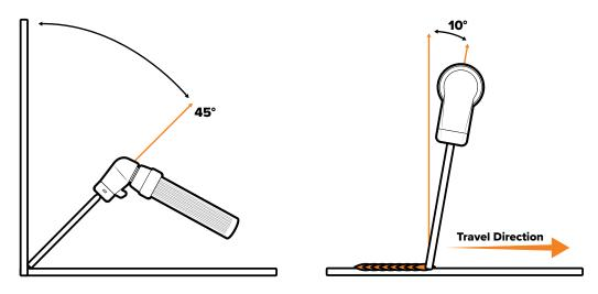
As you weld, keep your arc length short. A good rule of thumb is that your arc length shouldn't be longer than your electrode diameter. If you're using a 2.6mm electrode, your arc length shouldn't be longer than 3mm. However, you don't want to be so close that your electrode is touching the metal, as it will stick. If you pull away too far, your arc will become unstable, you'll produce more spatter, which will fly everywhere, and it'll become hard to keep the arc lit.
