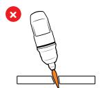
Torch angled to the material. Unequal bevel, one side may be excessively bevelled.
