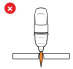
Torch height too low. Reverse bevel. The tip may contact the work and short out or damage the tip.
