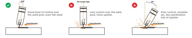
For example, say you're welding in a fillet joint (a corner join) with a standard steel wire. Your torch will be angled into it at a 45° angle, and then you'll angle slightly to the side (in a push direction) so that your gas can cover the weld pool and in front of the weld as you go.
